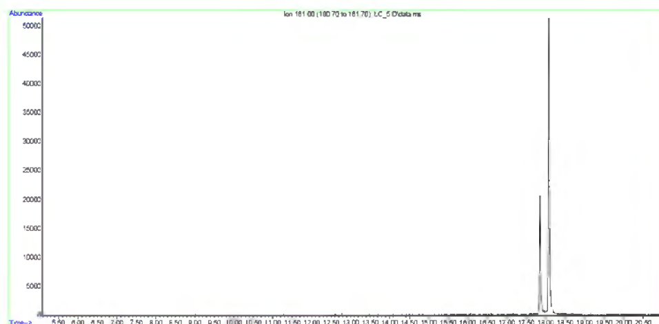
Figure 2 - Chromatogram, retention time and spectrum of the calibration solution of lambda-cyhalothrin (C = 10 µg/ml)
